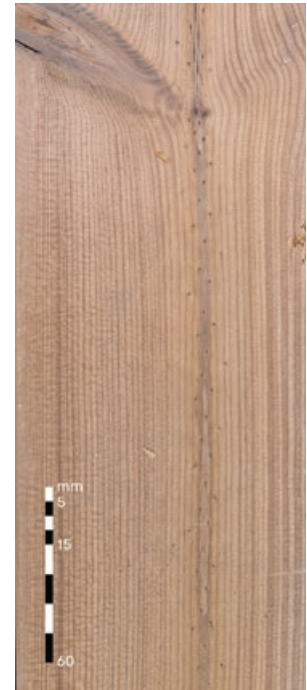
Sound heartwood A grade: Allowed, unlimited B grade: Allowed, unlimited
