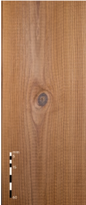
Sound knots A grade: Allowed, unlimited B grade: Allowed, unlimited
