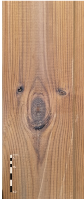
Knot cluster A grade: Allowed, unlimited B grade: Allowed, unlimited
