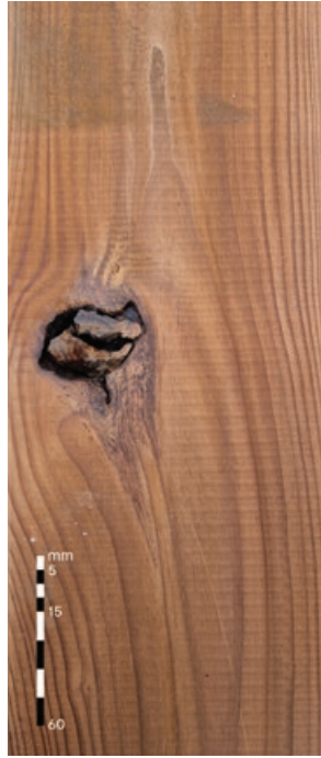
Cracked knots A grade: Allowed, up to 1/10 board width B grade: Allowed, unlimited
