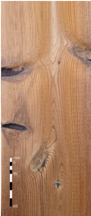
Knotholes on the sides A grade: Allowed, up to 15 mm wide B grade: Allowed, unlimited
