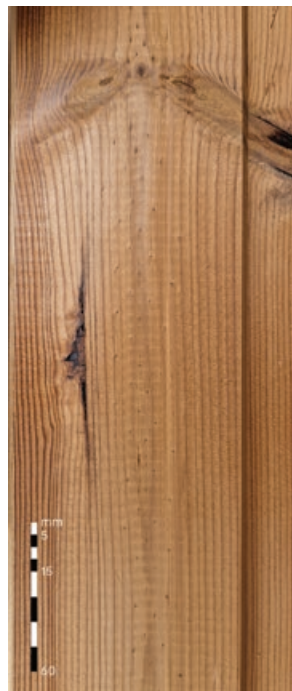
Resin pockets A grade: Allowed, up to 200 mm long B grade: Allowed, unlimited
