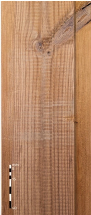
Feed-roller marks (from 0.5 mm deep) A grade: Not allowed B grade: Allowed, unlimited
