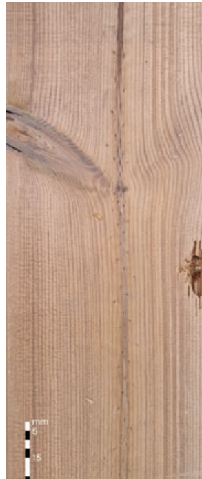
Mechanical defects A grade: Not allowed, except 80 mm ends of board B grade: Allowed, up to 300 mm long, max 0,5 pc. x board length, m
