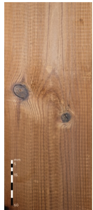
Knots with perimeter crack A grade: Allowed, up to \varnothing 20 mm B grade: Allowed, unlimited
