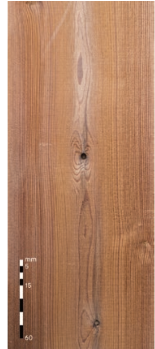
Dead black knots A grade: Allowed, up to 1/10 board width B grade: Allowed, unlimited
