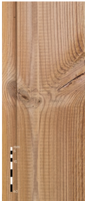
Knot shakes on the edges A grade: Allowed, up to 1/10 board width B grade: Allowed, unlimited
