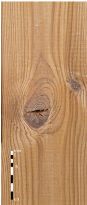
Knot shakes A grade: Allowed, up to 5 mm wide & 50 mm long B grade: Allowed, unlimited
